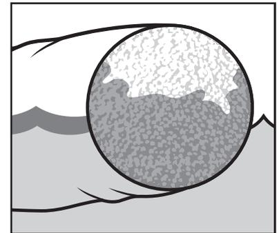
As the spill is absorbed, the boom floats lower in the water. Oil is now exposed to fresh absorbent.
