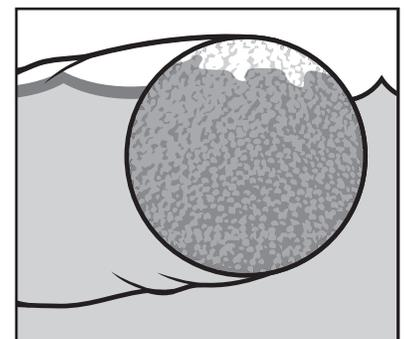
When completely saturated, the boom will 'bob' just below the water's surface. (Boom must now be replaced). Fluid stays absorbed, and retrieval is easy.
