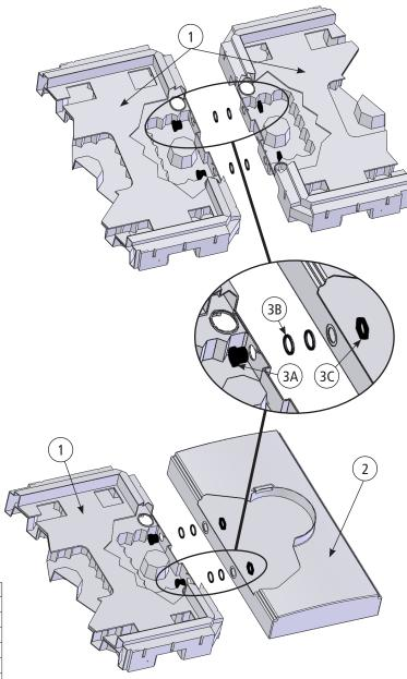
**NOTES:** All plug assemblies should be tight before putting product in use. Wrench and hole saw kit provided; portable drill and (2) % " drive ratchets not provided.
