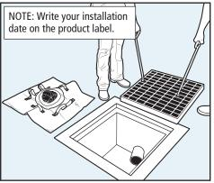
1. Remove drain grate and clean any sediment or debris from grate lip and ground surface.
