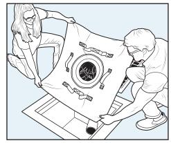
2. Place Drain Filter over opening. Filter fabric should overlap drain at least 7-8cm on all
