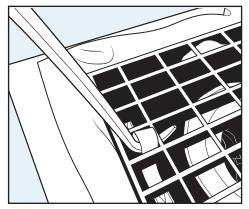
TIP: When it's time to empty or changeout your filter, remove the grate and filter at the same time by feeding grate hook through hi-viz strap before lifting.
