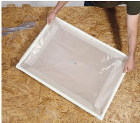
5. Flip assembled diverter over with legs down on flat surface and adjust until unit is level.
