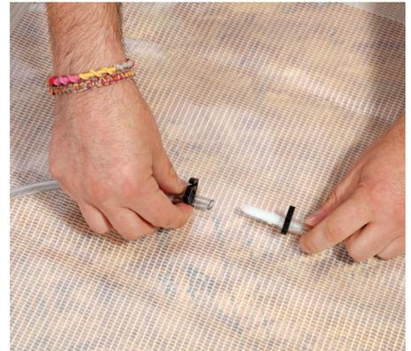
3. Locate enclosed barbed fitting and 2 hose clamps. Slide one clamp onto the hose and the other clamp onto drain valve that is attached to the diverter. Push the barbed fitting into end of hose and drain valve until secured into place.
