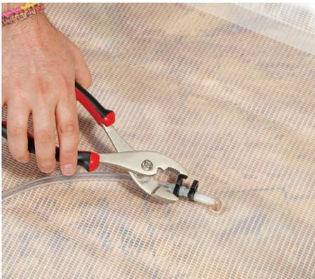
4. Slide clamps over the barbed fitting and pinch together with pliers to secure the clamp onto the hose and fitting.
