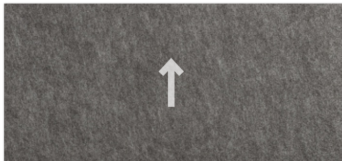
23cm x 56cm sample after 100,000 vertical steps shows no significant pile disturbance or degradation
